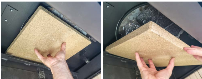
Removal of upper deflector plate
