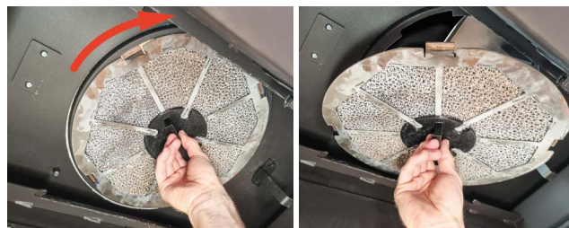
Loosening and removing the catalytic converter unit with the accessory tool
